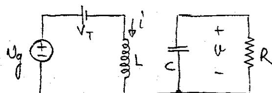
$$L \frac{di}{dt} = U_g - V_T \Rightarrow \frac{di}{dt} = \frac{U_g}{L} - \frac{V_T}{L}$$
