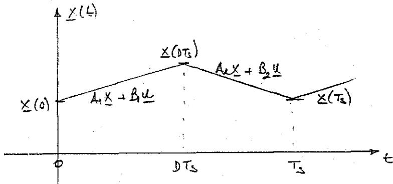
The same arguments apply during the second interval. With the switch in position 2, we have
