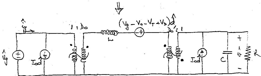
Complete ac small-signal model for the buck-boost converter
