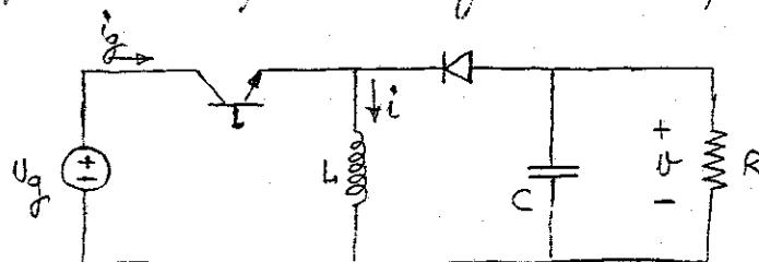
Include effects of transistor and diode voltage drops  $V_T$  and  $V_D$
