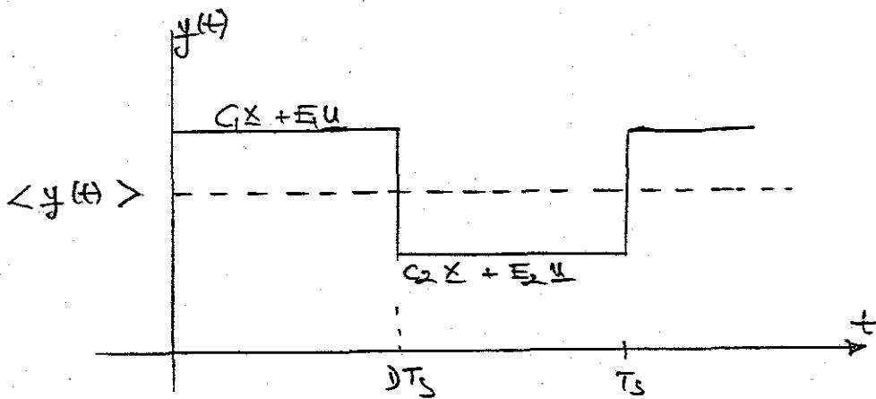
If  $G \neq C_2$  or  $E_1 \neq E_2$ , then  $y(t)$  may not be a continuous function of time; we are interested in the low frequency components of  $y(t)$  (much less than
