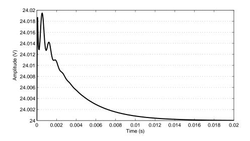
Figure 13.8: Unit step $v_g$  response of Ćuk converter - MRROLQGI/LTR compensator
