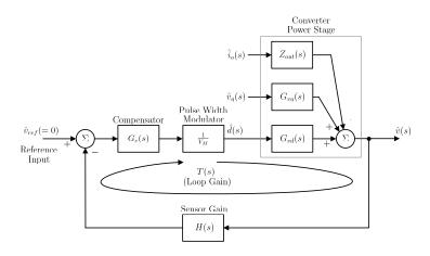
Figure 4.1: Generalized Power System Model
