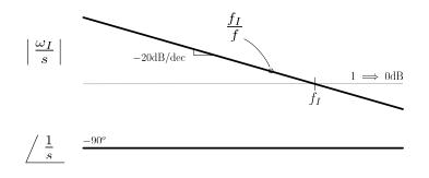
Figure 4.8: Bode Plot of Dominant Pole Compensator
