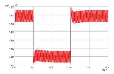
Figure 6.18: PECS Simulation of Active Droop Compensated Response to a Load Current Step
