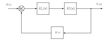
Figure 5.8: Feedback System Block Diagram
