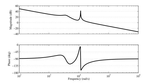
Figure 10.5: Loop gain of Ćuk converter controlled by FSFBI.
