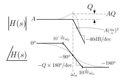
Figure 3.7: Second Order Complex Pole at  $\omega_o$
