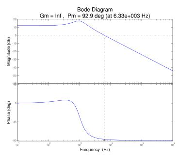
Figure 6.5: MATLAB Bode Plot of Loop Gain with Passive Droop Compensation
