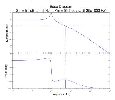
Figure 4.26: Matlab Lead Compensator
