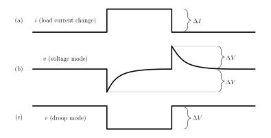
Figure 6.1: Transient Response of System with Droop Control
