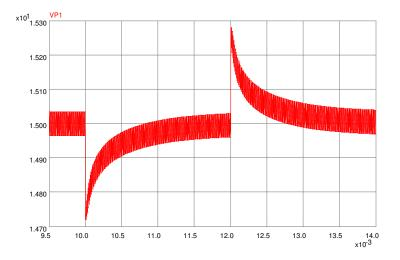
Figure 6.28: PECS Simulation of Voltage Mode Compensated Response to a Load Current Step
