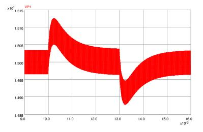
Figure 6.29: PECS Simulation of Voltage Mode Compensated Response to a Supply Voltage Disturbance
