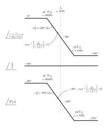
Figure 4.9: Graphical Construction of Phase Asymptotes for Dominant Pole Compensated Open Loop
