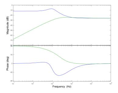
Figure 6.25: MATLAB Bode Plot of  $\mathbb{Z}_o$  for Voltage Mode Compensated System
