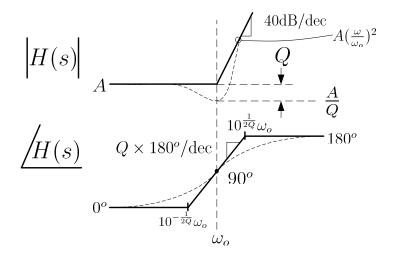
Figure 3.8: Second Order Complex Zero at  $\omega_o$
