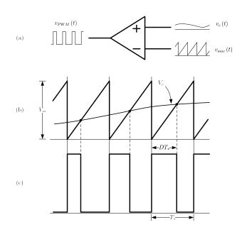
Figure 2.11: PWM Conversion Diagram
