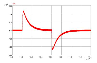
Figure 4.40: PECS Simulation of Lead Compensated System with Zero at 150Hz
