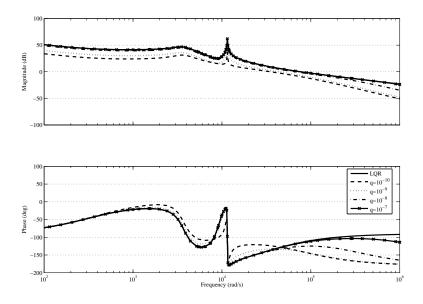
Figure 13.6: Loop transfer recovery of a ROKF-based LQGI compensator.
