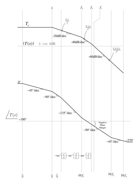
Figure 5.9: Bode Plot: Uncompensated System
