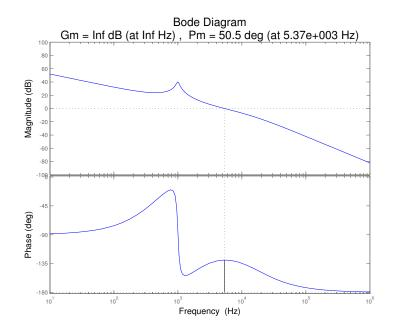
Figure 4.32: Matlab Lead Compensator with Integrator and Zero at 500Hz
