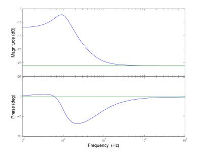
Figure 6.6: MATLAB Bode Plot of  $Z_o$  for Passive Droop Compensated System
