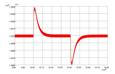
Figure 4.35: PECS Simulation of Lead Compensated System with Zero at 500Hz
