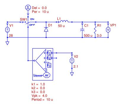
Figure 4.6: PECS Schematic of Open Loop System
