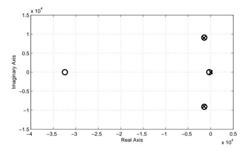
Figure 13.2: Compensator pole-zero plot showing likely pole-zero pair cancellation.
