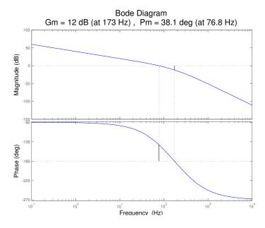
Figure 5.18: Matlab Analysis of Dominant Pole Compensated System with Zero
