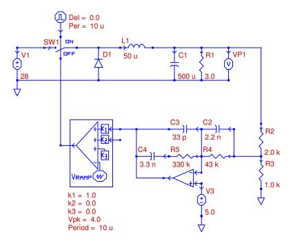
Figure 4.39: PECS Schematic of Lead Compensated System with Zero at 150Hz
