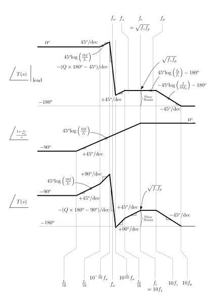
Figure 4.30: Bode Plot of Lead Compensator (500Hz)
