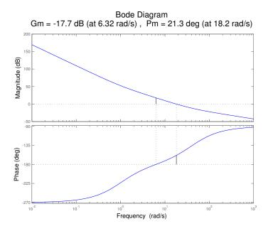
Figure 5.2: Matlab Analysis of phase and gain margin
