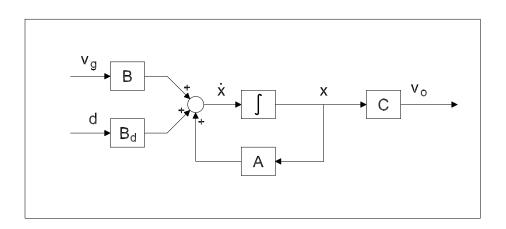
Figure 8.2: State space model of the Cuk converter.
