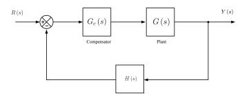
Figure 2.1: Feedback System Block Diagram
