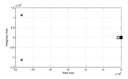
Figure 13.1: Pole-zero plot of the LQGI/LTR compensator.
