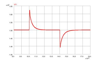
Figure 4.18: PECS Simulation of Dominant Pole with Zero Compensation and Damping
