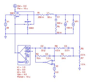
Figure 6.27: PECS Schematic of System with Voltage Mode Compensation
