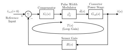
Figure 2.3: Simplified System Diagram
