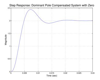
Figure 5.22: Step Response of the Dominant Pole with Zero Compensated System
