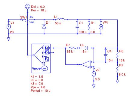
Figure 4.43: PECS Schematic of Extended System
