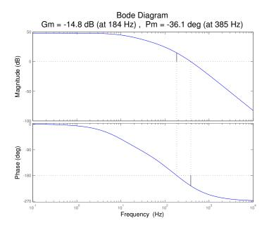
Figure 5.10: Matlab Analysis of Uncompensated System
