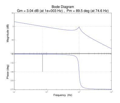
Figure 4.12: Matlab Analysis of Dominant Pole Compensator
