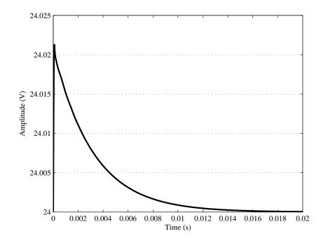
Figure 12.4: Unit step disturbance response of Ćuk converter controlled by LQG compensator.
