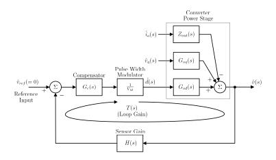
Figure 2.4: Generalized Power System Model
