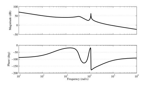
Figure 12.2: Loop gain of Ćuk converter controlled by LQR compensator.
