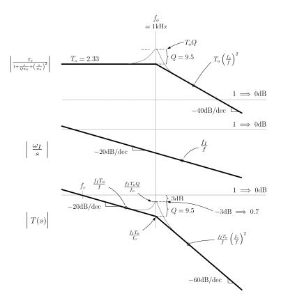
Figure 4.10: Graphical Construction of Gain Asymptotes for Dominant Pole Compensated Open Loop
