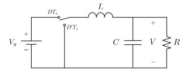
Figure 2.8: Ideal Buck Converter Circuit
