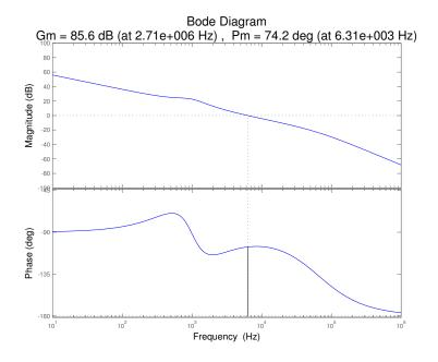
Figure 6.24: MATLAB Bode Plot of Loop Gains with Voltage Mode Compensation
