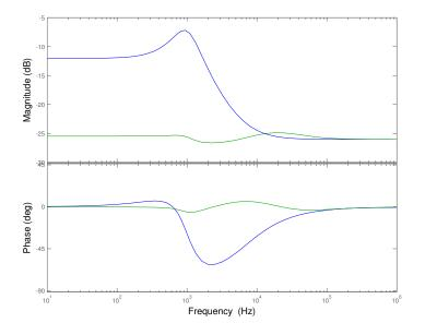
Figure 6.15: MATLAB Bode Plot of  $\mathbb{Z}_o$  for Active Droop Compensated System
