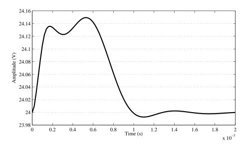
Figure 11.2: Unit step disturbance response of Ćuk converter with ESFBI compensator.
