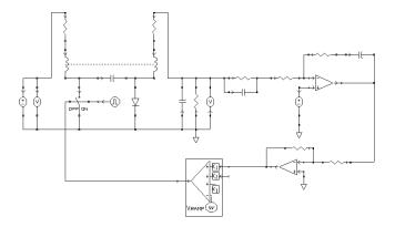
Figure 15.1: PECS simulation of Ćuk converter - MRROLQGI/LTR compensator.
