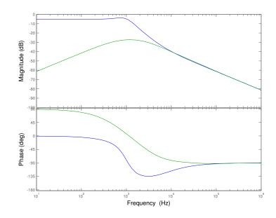
Figure 6.26: MATLAB Bode Plot of  ${\cal G}_{vg}$  for Voltage Mode Compensated System
