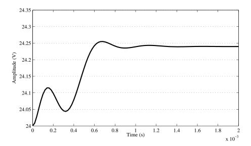
Figure 9.3: Response to unit step disturbance of input voltage.
