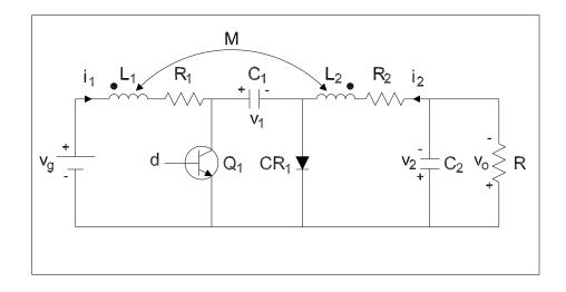
Figure 8.1: Cuk converter with inductor equivalent series resistances.
