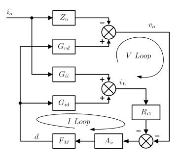
Figure 6.12: Small-signal block diagram of the current sensing mode
