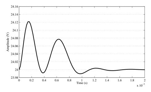
Figure 10.4: Unit step disturbance response of system with FSFBI controller.
