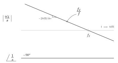
Figure 5.11: Bode Plot: Dominant Pole Compensator
