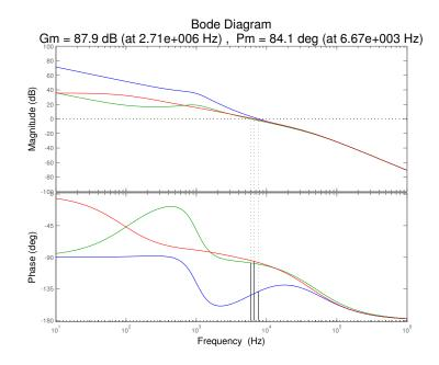
Figure 6.14: MATLAB Bode Plot of Loop Gains with Active Droop Compensation
