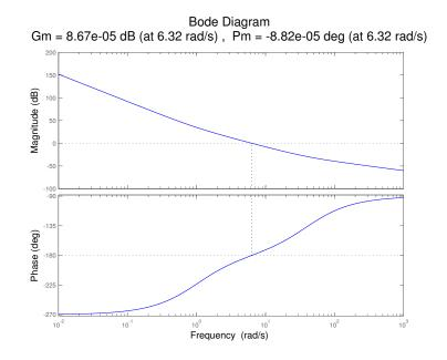
Figure 5.7: Matlab Analysis of phase and gain margin with parametric shift
