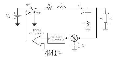
Figure 2.2: Buck Converter Circuit System Diagram
