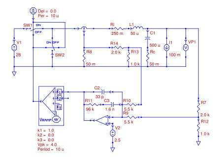
Figure 6.17: PECS Schematic of System with Active Droop Compensation
