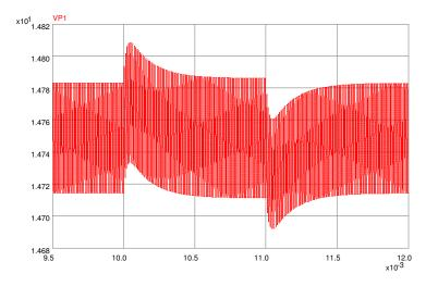
Figure 6.19: PECS Simulation of Active Droop Compensated Response to a Supply Voltage Disturbance
