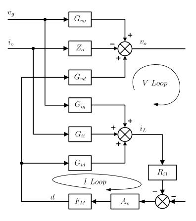
Figure 6.13: Small-signal block diagram of the current sensing mode -General
