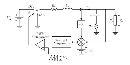
Figure 6.11: Buck converter with the current sensing mode [2]
