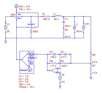
Figure 6.8: PECS Schematic of System with Passive Droop Compensation
