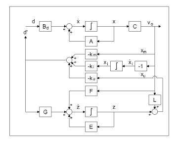
Figure 13.5: Loop transfer recovery with a reduced-order observer.
