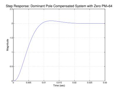
Figure 5.24: Step Response of the Dominant Pole with Zero Compensated System (Improved Margin)
