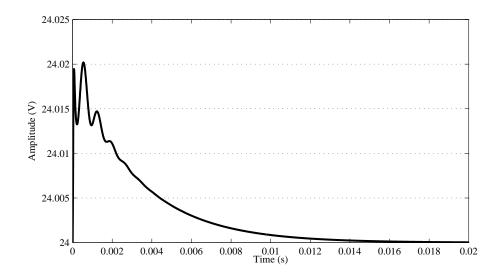
Figure 13.4: Unit step disturbance response of Ćuk converter - MRLQGI/LTR compensator.
