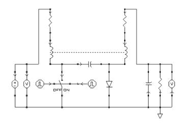
Figure 8.4: The Ćuk converter simulated in PECS.
