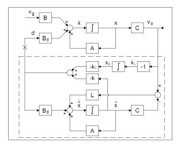
Figure 11.1: An estimated state feedback compensator with integral action.
