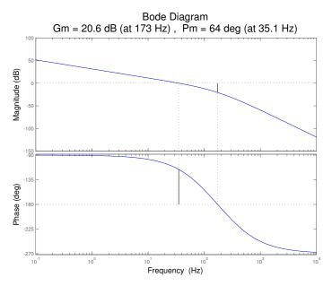
Figure 5.23: Matlab Analysis of Dominant Pole Compensated System with Zero (Improved Margin)
