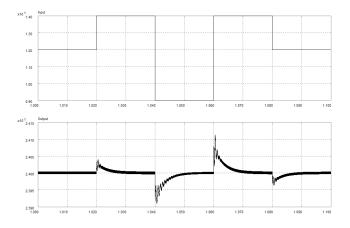
Figure 15.3: Large signal  $v_g$  disturbances and  $v_o$  response - MRROLQGI/LTR compensator.
