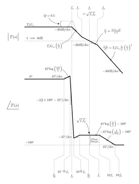
Figure 4.25: Bode Plot of Lead Compensated System
