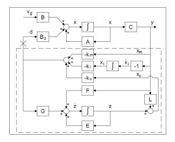
Figure 11.6: A state feedback regulator with integral action based on a reduced-order estimator.
