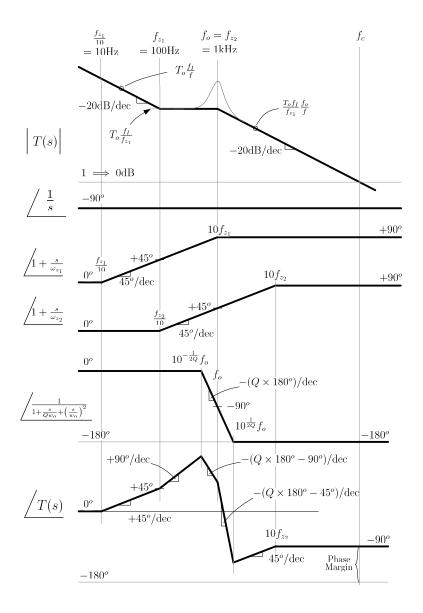
Figure 4.41: Extended Bandwidth Bode Plot and Phase Construction
