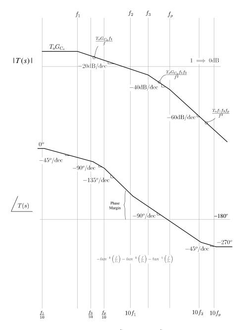
Figure 5.27: Lead Compensated System
