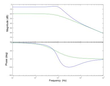
Figure 6.7: MATLAB Bode Plot of  $G_{vg}$  for Passive Droop Compensated System
