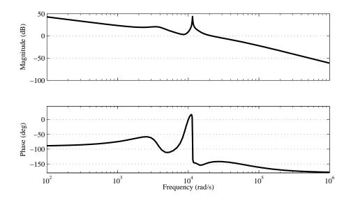
Figure 11.8: Loop gain of Ćuk converter controlled by ROESFBI compensator.
