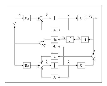
Figure 12.8: The loop to be recovered during loop transfer recovery with a full-order observer.
