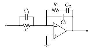
Figure 4.33: Compensator Circuit for Dominant Pole with Lead Compensation
