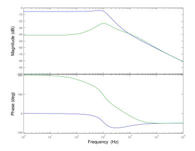
Figure 6.16: MATLAB Bode Plot of  ${\cal G}_{vg}$  for Active Droop Compensated System
