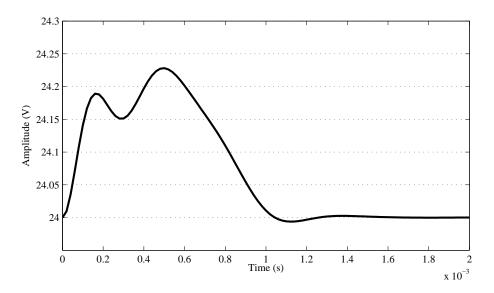
Figure 11.7: Unit step disturbance response of Ćuk converter with ROESFBI compensator.
