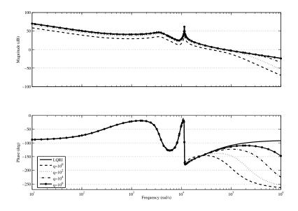
Figure 12.9: Loop transfer recovery of an LQGI compensator.
