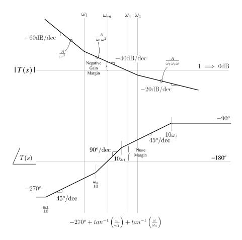
Figure 5.1: Bode Plot: System Loop Gain
