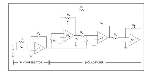
Figure 14.1: The MRLQGI/LTR compensator implemented using operational amplifiers.
