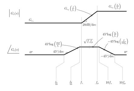
Figure 4.24: Bode Plot of Lead Compensator
