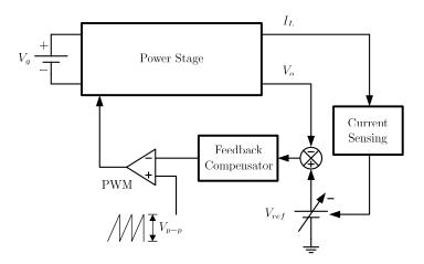
Figure 6.2: Active Droop Control System Block Diagram
