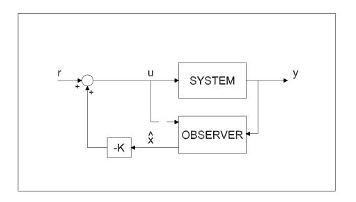
Figure 12.7: Input decoupling effect of loop transfer recovery.
