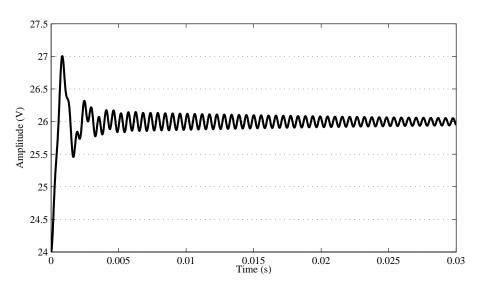
reject disturbances on the input voltage  $v_g$ . Also, note that the output of the circuit is a lightly damped sinusoid, with an approximate frequency of 1.83 kHz (11.5 krad/s).
