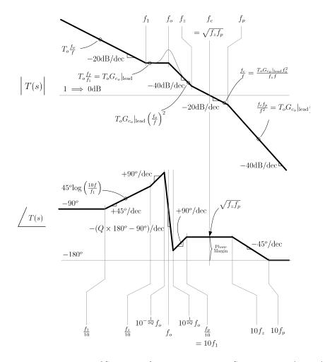
Figure 4.37: Bode Plot of System with Lead plus Integral Compensation (150Hz)
