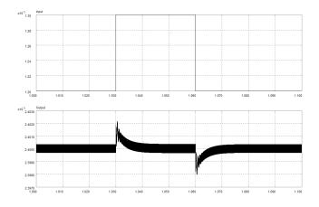
Figure 15.2: Unit step  $v_g$  disturbances and  $v_o$  response - MRROLQGI/LTR compensator.
