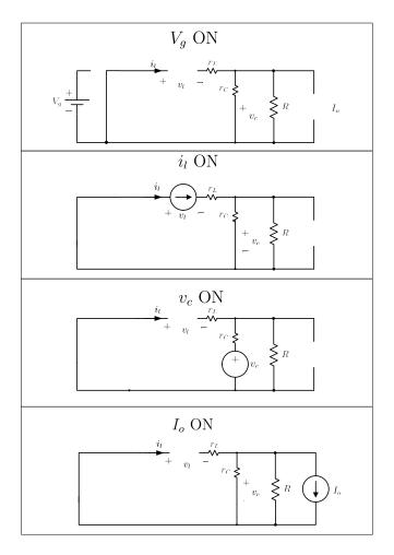
Figure 2.7: Buck Converter Superposition Analysis: D'Ts
