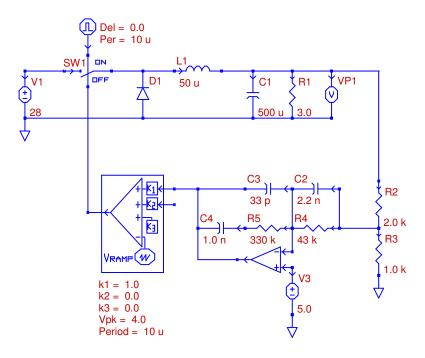
Figure 4.34: PECS Schematic of Lead Compensated System with Zero at 500Hz
