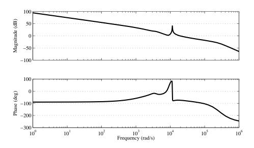
Figure 11.3: Loop gain of Ćuk converter controlled by ESFBI compensator.
