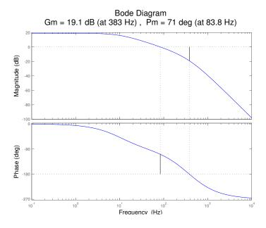
Figure 5.28: Matlab Analysis of Lead Compensated System
