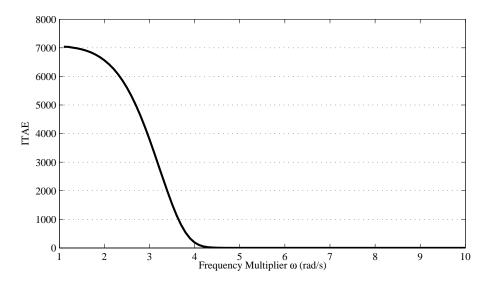
The frequency multiplier was swept and the minimum ITAE determined to occur at  $\omega = 6.564$  rad/s. The step disturbance transient is shown in Figure 10.4. The
