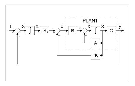
Figure 10.1: Generic system controlled with a FSFB regulator and output integral feedback.
