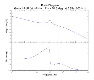
Figure 4.38: Matlab Lead Compensator with Integrator and Zero at 150Hz
