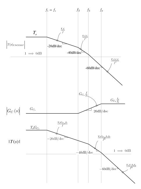
Figure 5.26: Lead Compensation Magnitude Construction
