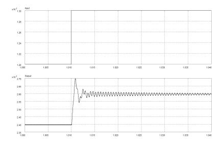
Figure 8.5: Unit step response of the Ćuk converter in PECS.
