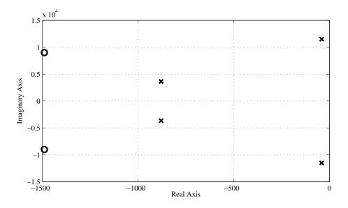
Figure 8.6: Map of the pole and zero locations of  $T_{v_o v_g}$ .
