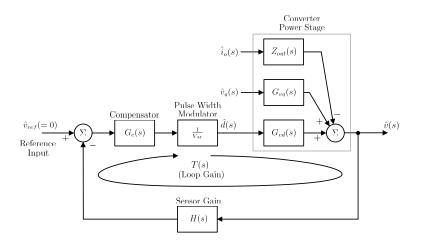
Figure 6.4: Buck converter control loop
