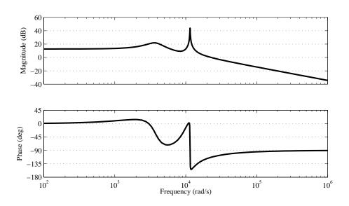
Figure 9.4: Loop gain with the full state feedback controller.
