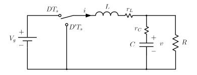
Figure 2.9: Buck Converter Circuit with Non-Ideal Circuit Elements
