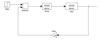
Figure 5.16: Simulink schematic of the Compensated System
