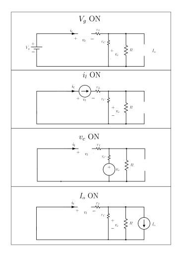
Figure 2.6: Buck Converter Superposition Analysis: DTs
