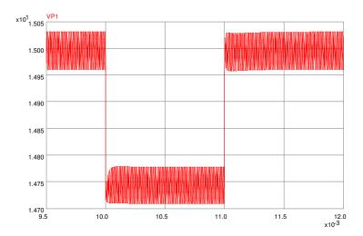
Figure 6.9: PECS Simulation of Passive Droop Compensation Response to a Load Current Step
