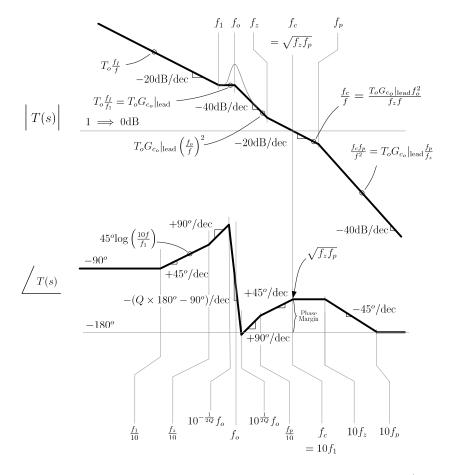
Figure 4.31: Bode Plot of System with Lead plus Integral Compensation (500Hz)
