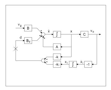
Figure 10.2: System controlled with a FSFBI regulator.
