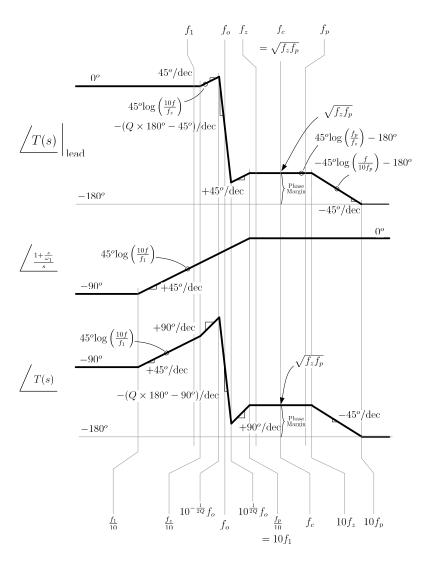
Figure 4.36: Bode Plot of Lead Compensator (150Hz)
