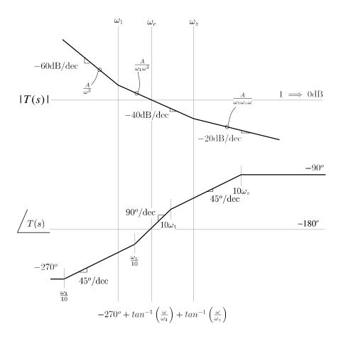
Figure 5.6: Bode Plot: System Loop Gain with parametric shift
