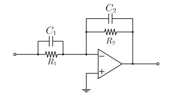
Figure 4.27: op-amp circuit implementation of lead compensator
