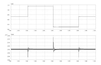
Figure 15.4: Load current disturbance and  $v_o$  response - MRROLQGI/LTR compensator.
