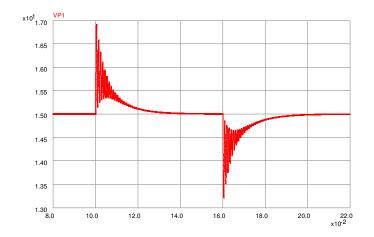
Figure 4.23: PECS Simulation of Dominant Pole with Zero Compensation (10 dB GM)  $\,$
