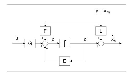
Figure 11.5: Reduced-order estimator construction.
