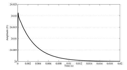
Figure 12.1: Unit step disturbance response of the Ćuk converter controlled by LQR.
