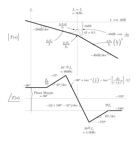
Figure 4.19: Open Loop System Gain and Phase with pole-zero Compensation (10dB GM)
