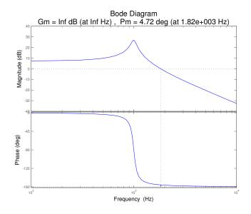
Figure 4.5: Matlab Uncompensated Bode plot
