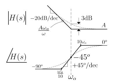
Figure 3.10: Inverted Zero at  $\omega_o$
