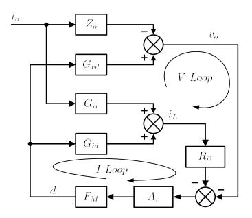
Figure 6.20: Complete Small-signal block diagram of the current sensing mode
