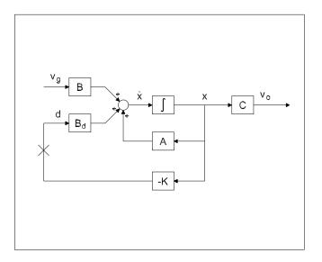
Figure 9.5: The full state feedback controller applied to the Ćuk converter.
