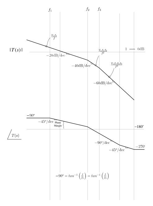
Figure 5.20: Dominant Pole with Zero Compensated System
