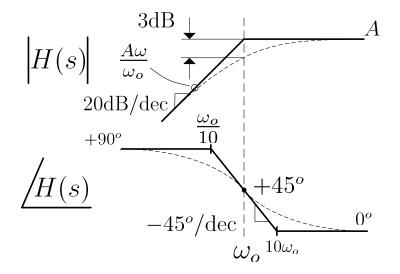
Figure 3.9: Inverted Pole at  $\omega_o$
