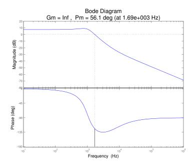
Figure 6.3: MATLAB Uncompensated Bode plot
