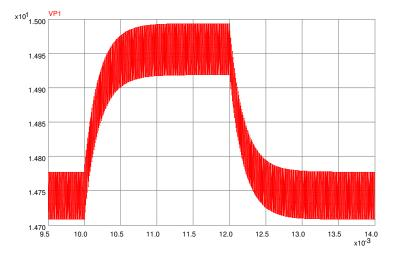
Figure 6.10: PECS Simulation of Passive Droop Compensation Response to a Supply Voltage Disturbance
