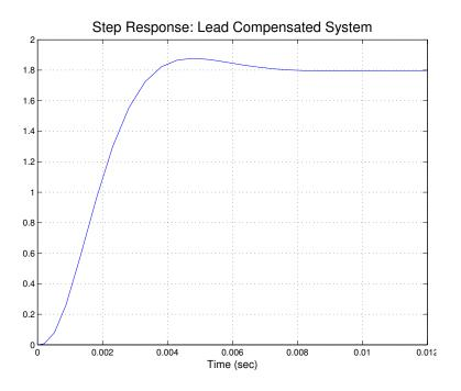
Figure 5.29: Step Response of the Lead Compensated System
