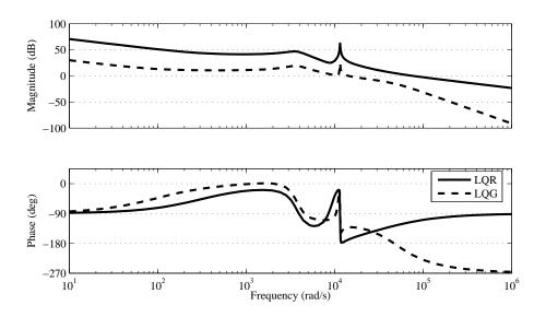
Figure 12.5: Loop gain of Ćuk converter controlled by LQR vs. LQG.
