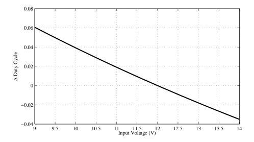
Figure 8.7: The small-signal duty cycle required over the full input voltage range to maintain nominal output voltage.
