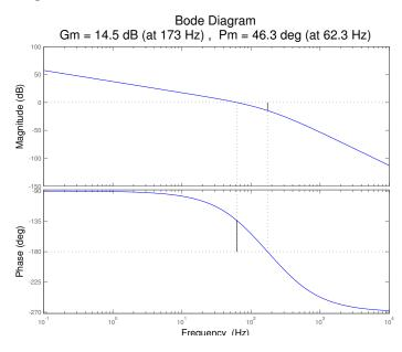
Figure 5.21: Matlab Analysis of Dominant Pole Compensated System with Zero
