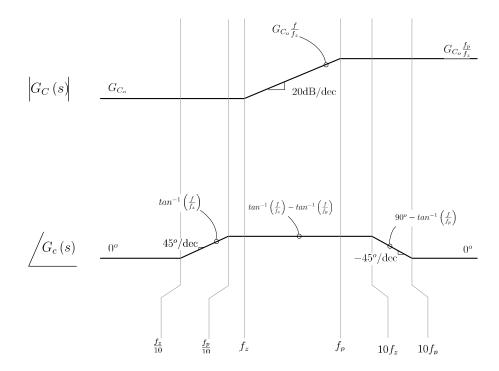
Figure 5.25: Bode Diagram: Lead Compensator
