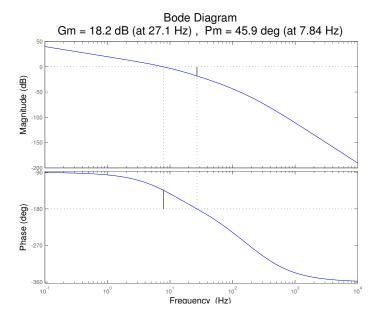
Figure 5.15: Matlab Analysis of Dominant Pole Compensated System
