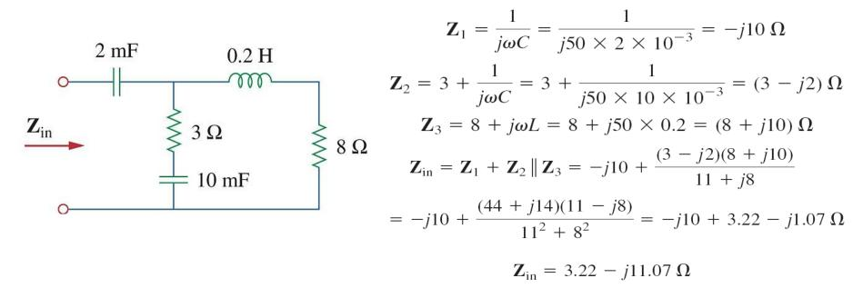
**Example:** Determine the input impedance at  $\omega = 10$  rad/s.
