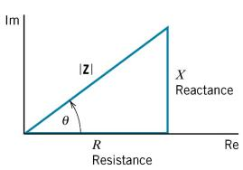
where  $R = \text{Re}(\mathbf{Z})$  is the resistance and  $X = \text{Im}(\mathbf{Z})$  is the reactance. Positive X is for L (or lagging) and negative X is for C (or leading).
