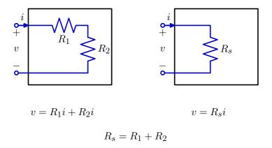
The resistance of a series combination is always **larger** than either of the original resistances.
