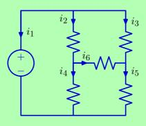
The number of independent KCL equations is one less than the number of nodes.
