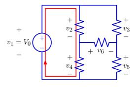
Example:  $-v_1 + v_2 + v_4 = 0$  or equivalently  $v_1 = v_2 + v_4$ .
