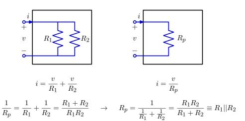
The resistance of a parallel combination is always **smaller** than either of the original resistances.
