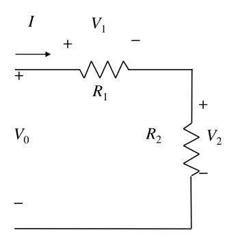
$$V_1 = \frac{R_1}{R_1 + R_2} V_0$$
