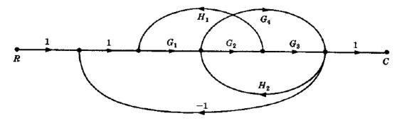
The two forward path gains are  $P_1 = G_1G_2G_3$  and  $P_2 = G_1G_4$ . The five feedback loop gains are  $P_{11} = G_1G_2H_1$ ,  $P_{21} = G_2G_3H_2$ ,  $P_{31} = -G_1G_2G_3$ ,  $P_{41} = G_4H_2$ , and  $P_{51} = -G_1G_4$ . Hence
