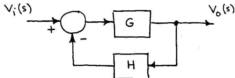
The feedback transmittance is determined by the resistors
