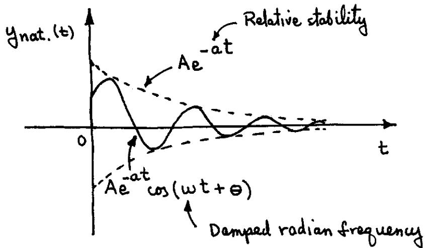
The character of the natural response component of a system can be determined by graphing the characteristic roots of its transfer function.
