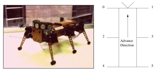
Figure 2: The Genghis II six-legged robot and its schematic top view.
