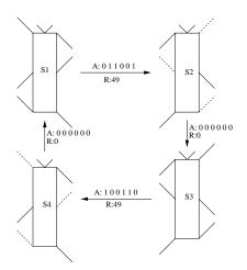
Figure 3: In the tripod gait four different situations are encountered and only three different actions are used. In the figure, dashed legs stand for legs in the air after performing a step. Observe that action A: 000000 always gets reward 0 and so its evaluation must be based on the future rewards it allows to obtain.
