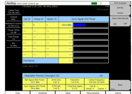
Over-the-Air Measurements – Sync Signal Power Too many strong sectors at the same location creates co-channel interference. This leads to low data rate, low capacity, and excessive soft handoffs.
