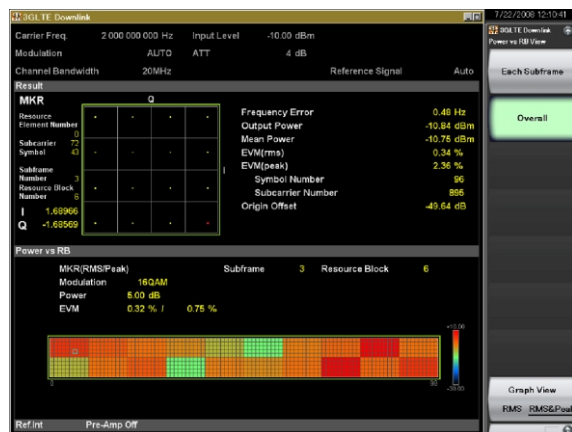
Figure 12: LTE analysis includes constellation analysis and graphical displays with resolutions of Subcarriers, Symbols, and Resource Blocks.
