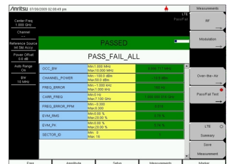
Pass/Fail Test Set up common test limits, or sets of limits, for each instrument. Inconsistent settings between base stations, leads to inconsistent network behavior.
